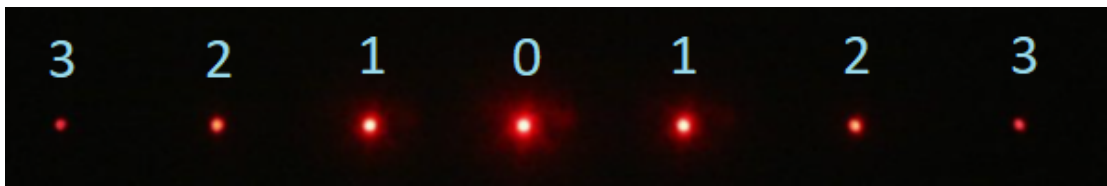
Figure 3.10: Interference pattern of laser light
